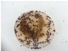
“Heavy Fraction” - glass beads and mud at the bottom of the Bowl after 4 flotations
